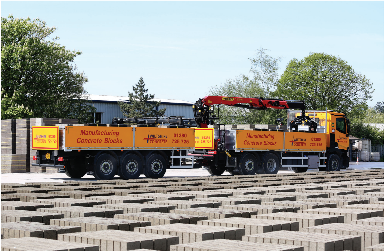
One of Wiltshire Concrete's five new C460 6x2 rigid block grabs with flatbed body and Palfinger crane plus VGB towing hook
